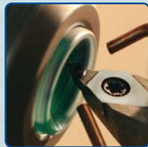
The aspheric base curve is cut first. The semi-finished lens is then turned around and the front curve is cut next.
